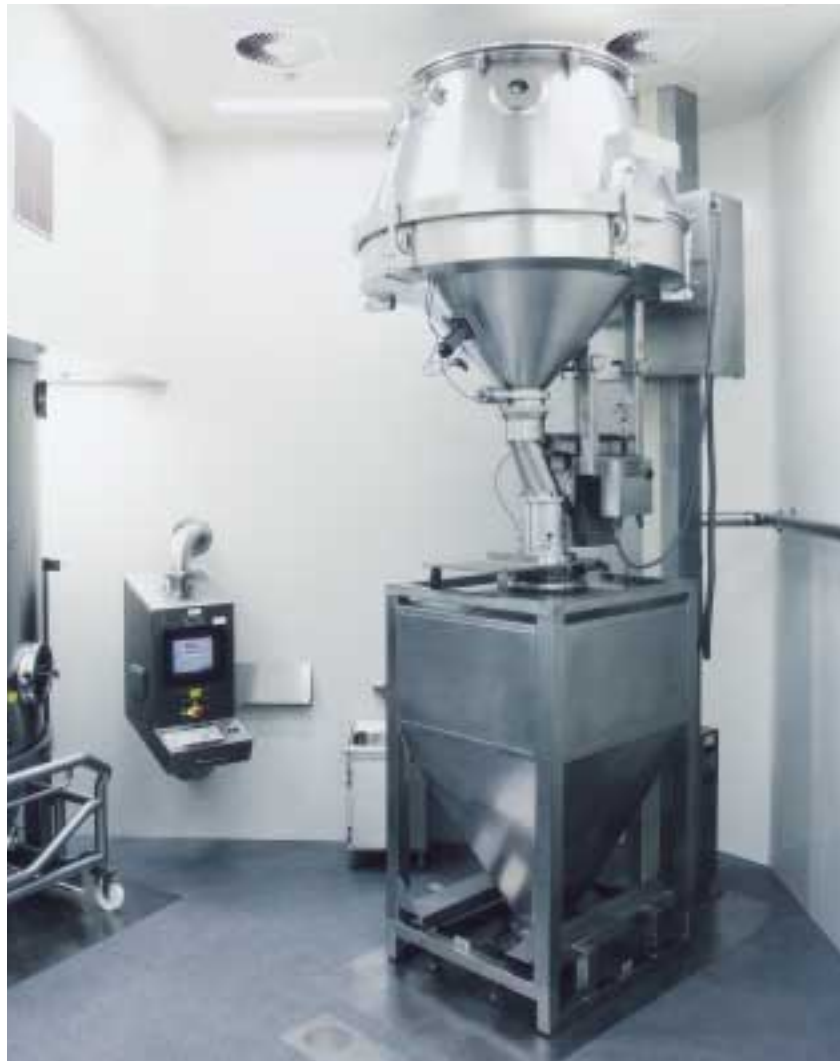
Sizing of granulates after fluid bed processing using the rotor mill GS 180
